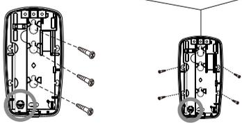
Set circuit board alignment post in position "0" or "1" to select mounting height.
