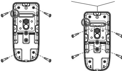
Set circuit board graduation in position "2.3m" or "3m" or "4m" to select mounting height. Tighten PCB mounting screws.
