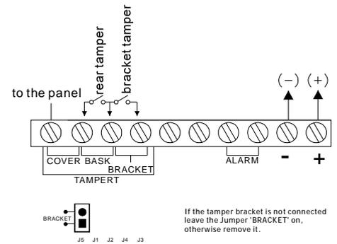
If the tamper bracket is not connected leave the Jumper 'BRACKET' on, otherwise remove it.
